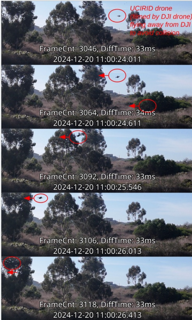
Fig. 10. Screenshots of video taken from DJI drone as it was flown towards UCIRID drone. The UCIRID takes collision avoidance action when the DJI drone breaches the predefined 30 m perimeter.
