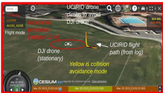
Fig. 11. Flight demonstration of collision avoidance. The UCIRID drone flies towards the stationary DJI drone. When the collision perimeter is breached, the UCIRID drone climbs to avoid collision.
