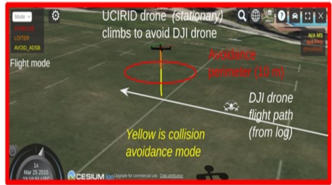
Fig. 12. Flight demonstration of collision avoidance. The UCIRID drone flies towards the stationary DJI drone. When the collision perimeter is breached, the UCIRID drone climbs to avoid collision.
