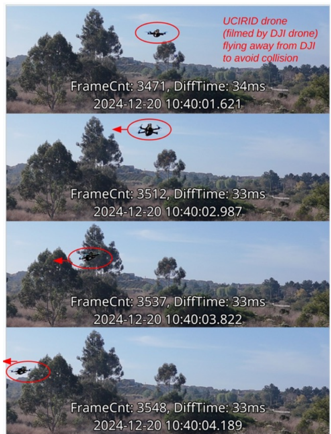
Fig. 9. Screenshots of video taken from DJI drone as it was flown towards UCIRID drone. The UCIRID takes collision avoidance action when the DJI drone breaches the predefined 10 m perimeter.
