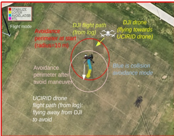
Fig. 8. Flight demonstration of collision avoidance. The UCIRID drone was in stationary mode, and the DJI drone flew towards it. Upon breach of the bubble, the UCIRID drone took autonomous collisions avoid action, flying away from the DJI drone.
