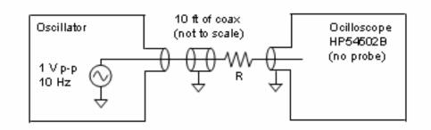
For the following, be careful: You need to take into account the scope input impedance, which forms a voltage divider with R. (The oscillator has zero output impedance. The voltage indicated is the actual voltage generated by the oscillator.)
