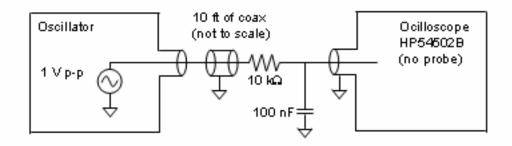
(The oscillator has zero output impedance. The voltage indicated is the actual voltage generated by the oscillator.)
