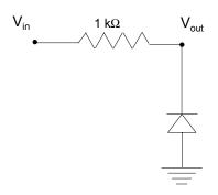
For this circuit,  $V_{in} = +10$  V.
