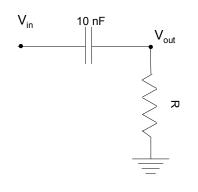
$$\frac{V_{out}}{V_{in}} = \frac{\omega RC}{\sqrt{1 + (\omega RC)^2}} = 0.71$$
