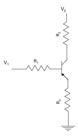
Assuming the transistor is in active mode, find the following quantities in term of  $R_1$ ,  $R_2$ ,  $R_3$ ,  $V_1$ , and  $V_2$ .
