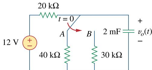
When the switch is at position A, the circuit reaches steady state. By voltage division,
