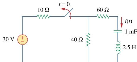
$$\text{At } t = 0, \quad i(0) = 0, \quad V_C(0) = 40 \times 30 / 50 = 24 \text{ V}$$
