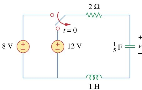
$$\text{At } t = 0^-, i_L(0) = 0, v(0) = v_C(0) = 8 \text{ V}$$
