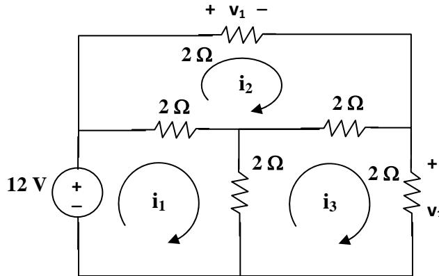
$$\text{For loop 1, } 12 = 4i_1 - 2i_2 - 2i_3 \text{ which leads to } 6 = 2i_1 - i_2 - i_3 \quad (1)$$
