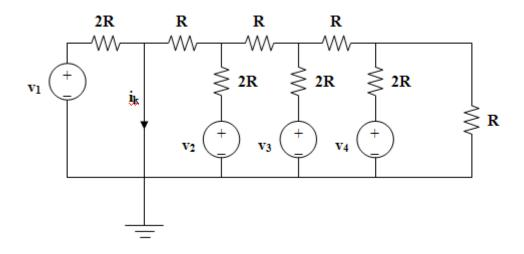
For the first case, let  $v_2 = v_3 = v_4 = 0$ , and  $i_1 = 1A$ .
