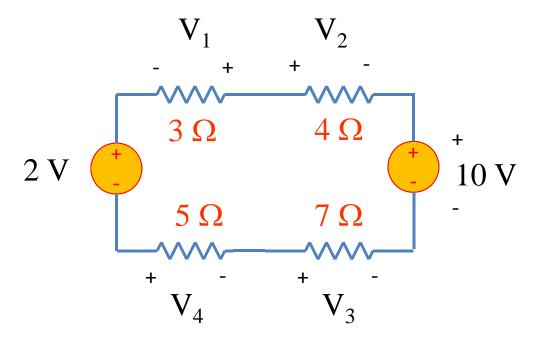
Problem 8: KVL, KCL & Ohm Find  $V_1$  through  $V_4$  and  $V_4$  and  $V_4$  in the circuit below.
