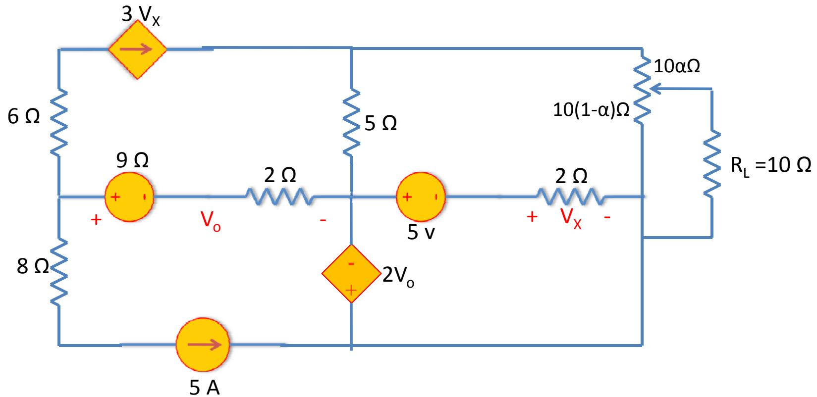
Problem 5) Find the maximum power transferred to  $R_L$ .  $[S]=[1/\Omega]$  is the unit for conductance.
