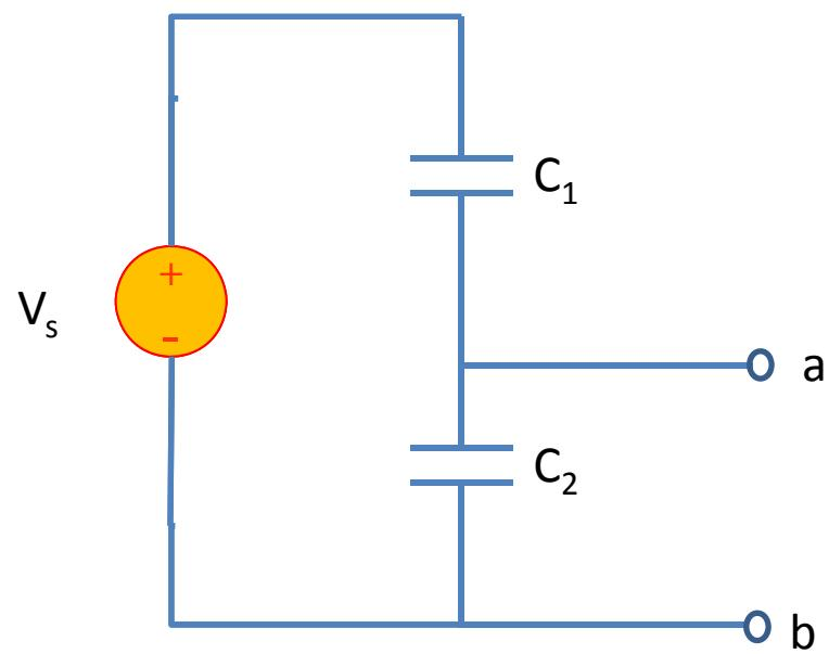
Problem 7) Find the equivalent capacitance. All Capacitors have the value of 1mF.
