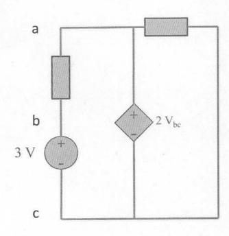
$$V_{ac} = 2V_{bc}$$
