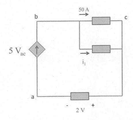
To find i:  $KCL \otimes node b$  5Vac = 50A + i Vac = -2V  $i_1 = 5(-2) - 50A$   $i_1 = -60A$
