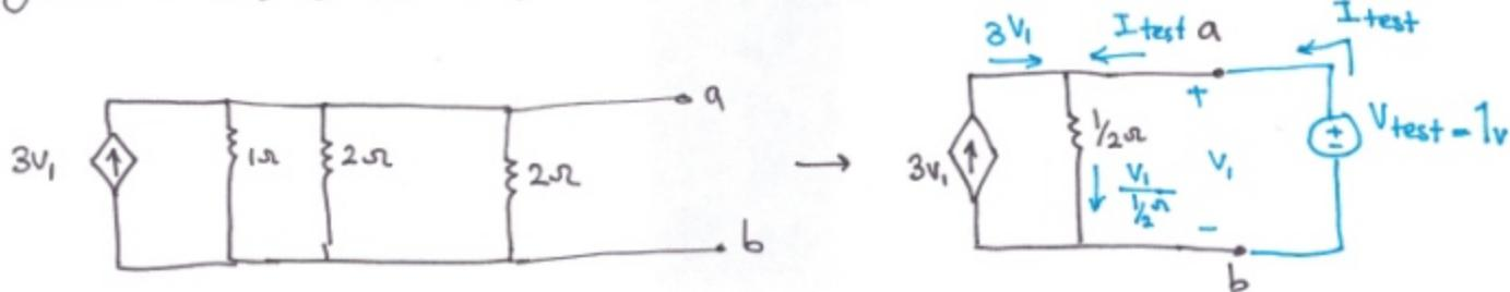
$$KCL: 3V_1 + I_{test} \neq \frac{V_1}{\frac{1}{2}\Omega}$$
