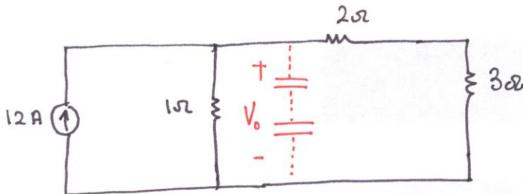
$$V_0 = 12 \times R_{eq} = 12 \times (1\Omega \parallel (2\Omega + 3\Omega))$$
