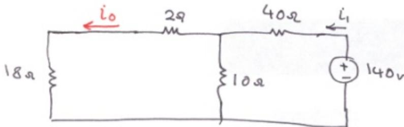
$$i_1 = \frac{140\text{v}}{40\Omega + (10||2+18)\Omega} = \frac{140\text{v}}{(40+10||20)\Omega} = 3\text{ A}$$
