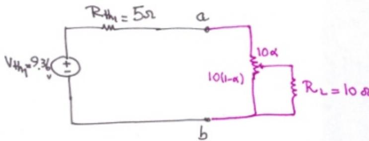
Step 2. Now we should find the equivalent circuit seen by  $R_L$ , we could have found this from the beginning, but it is easier to do it two steps:
