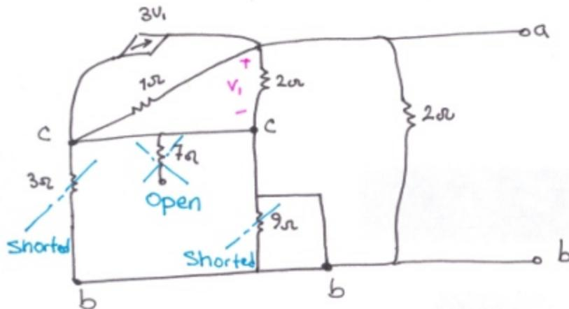
As you can see, when the  $1\Omega$  voltage source is turned off, terminals nodes (b) and (c) are shorted, so the  $9\Omega$  and the  $3\Omega$  resistors can be ignored (they are shorted), the  $7\Omega$  resistor is open and can be ignored, this is the simplified circuit diagram:
