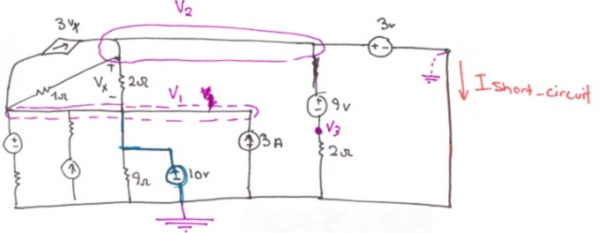
node 1:  $V_1 = 10V$  (because of the voltage source)
