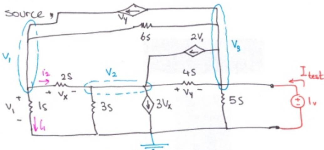
\* S is the unit for conductance ( $G$ ). So for example, the current flowing in the 1s conductance:
