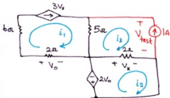
Here we can use nodal or mesh analysis to find  $V_{test}$ .
