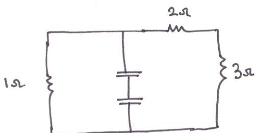
$$R_{eq} = 1\Omega \parallel (2\Omega + 3\Omega) = 5/6\Omega$$
