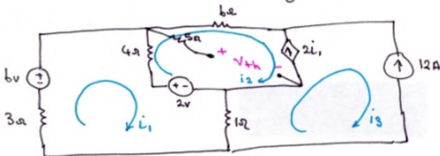
note that for the  $5\Omega$  resistor, since terminals a-b are open, there is no current flowing in the  $5\Omega$  resistor  $\Rightarrow$  can be neglected.
