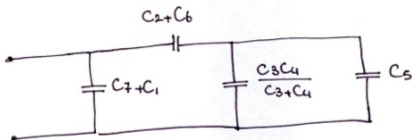
$$C_1 = C_2 = C_3 = C_4 = C_5 = C_6 = C_7 = 1 \text{ mF}$$
