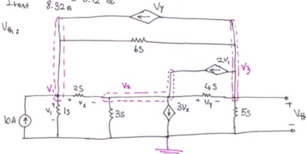
$$\text{Node 1: } 1 \cdot V_1 + 2(V_1 - V_2) + 6(V_1 - V_3) - V_y = 10 \text{ A}$$
