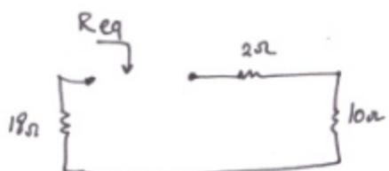
$$R_{eq} = 2\Omega + 8\Omega + 10\Omega = 20\Omega$$
