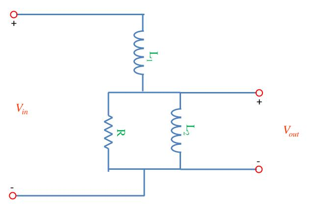
Calculate  $H(\omega)$  for this circuit. Sketch the magnitude of  $H(\omega)$  vs.  $\omega$ .
