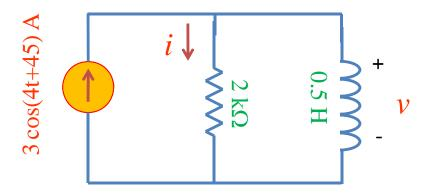
Find i(t) and v(t). Hint: convert the current source into a phasor, then find the current and voltage phasors for the whole circuit, then convert back to the time dependent i(t), v(t).
