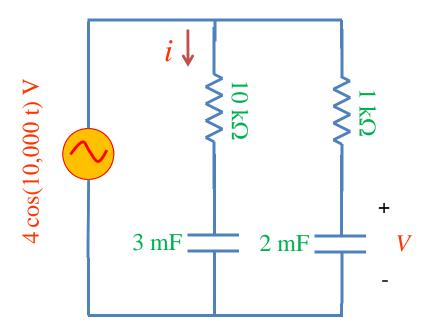
Find i(t) and v(t). Hint: convert the voltage source into a phasor, then find the current and voltage phasors for the whole circuit, then convert back to the time dependent i(t), v(t).
