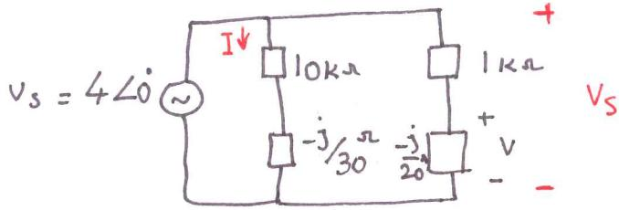
$$V = \frac{V_s \times Z_4}{Z_4 + Z_3} = \frac{4 \times -j/20}{(-5000 + j/4) \times 4} = \frac{4j}{-20000 + j} = \frac{4j}{-20000\sqrt{1 + 1/160000}} = \frac{4j}{-20000\sqrt{1.00000001}} = \frac{4j}{-20000} = -0.2 \angle -90^\circ \text{ V}$$
