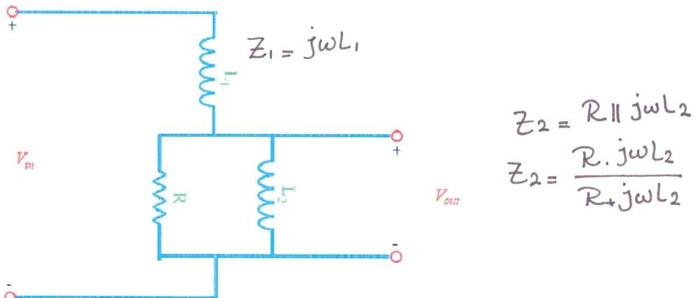
Calculate  $H(\omega)$  for this circuit. Sketch the magnitude of  $H(\omega)$  vs.  $\omega$ .
