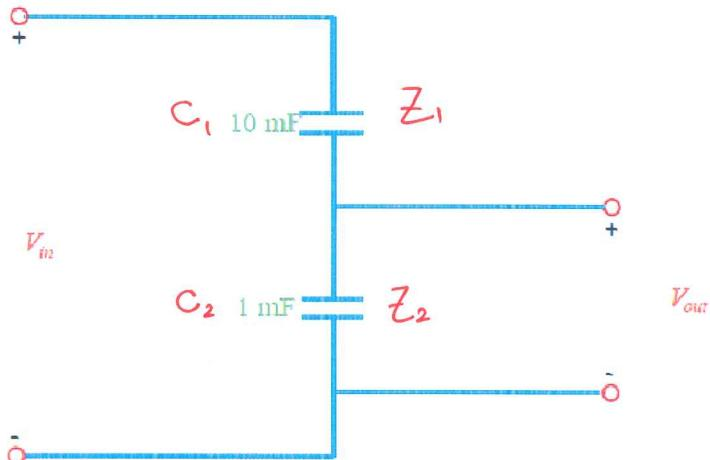
Calculate  $H(\omega)$  for this circuit. Sketch the magnitude of  $H(\omega)$  vs.  $\omega$ .
