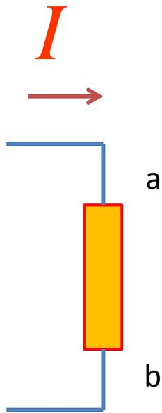
$$I \times V_{ab} = \text{power}$$
