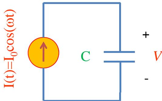
$$j \equiv \sqrt{-1} \quad q = CV \quad i = C \frac{dv}{dt}$$
