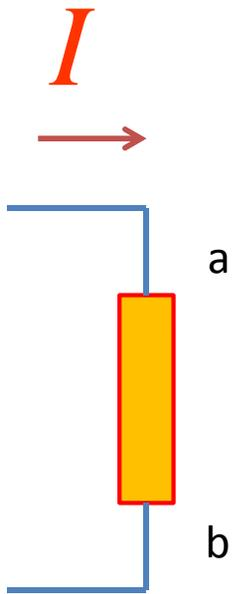
$$I \times V_{ab} = \text{power}$$
