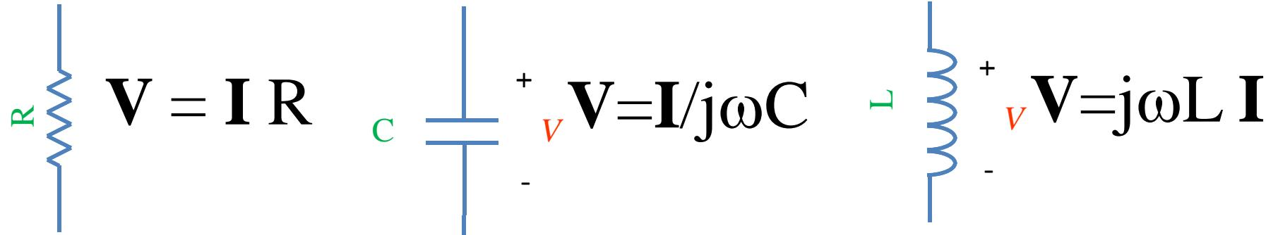
The diagram shows three circuit components: a resistor (R) represented by a blue zigzag line, a capacitor (C) represented by two vertical lines with a central gap, and an inductor (L) represented by a blue coil. To the left of each symbol is its corresponding voltage-current relationship equation.
