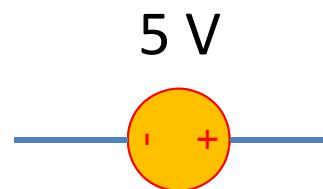
$$\text{Voltage drop} = - 5 \text{ V}$$
