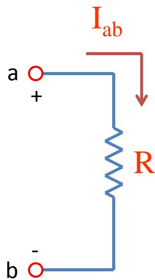
$$V_{ab} = I_{ab} \times R$$
