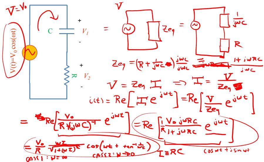
$$i(t) = \operatorname{Re} \left[ \frac{1}{R} \frac{V_{0,jw}(R)}{I + jwRC} e^{jwE} \right] = \frac{V_{0}}{R} \operatorname{Re} \left[ \frac{JwL}{I + jwL} e^{jwL} \right]$$
