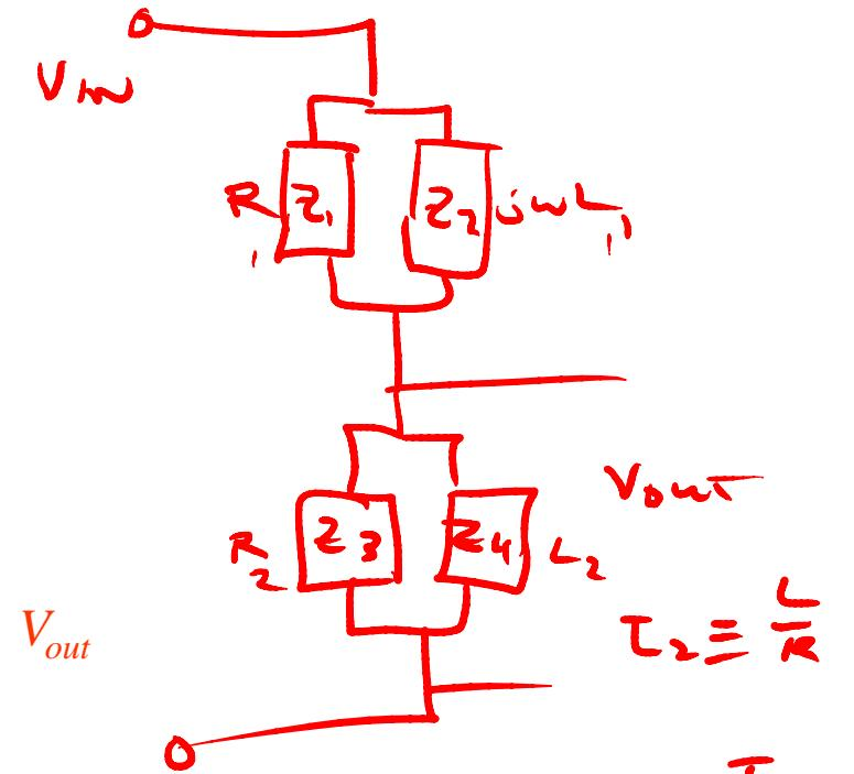
Calculate  $H(\omega)$  for this circuit. Sketch the magnitude of  $H(\omega)$  vs.  $\omega$ .
