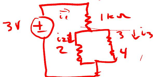
$$i_1 = \frac{3V}{1 + 2 \parallel (3+4) k\Omega} = \frac{3}{1 + 2 \parallel 7} \text{ mA}$$
