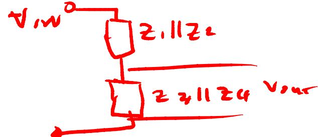
$$\begin{aligned} \frac{V_{out}}{V_{in}} &= \frac{(Z_3 \parallel Z_4)}{(Z_3 \parallel Z_4) + (Z_1 \parallel Z_2)} \\ H(\omega) &= \frac{\frac{j\omega L_2}{1+j\omega\tau_2}}{Z_1 \parallel Z_2 + \frac{j\omega L_1}{1+j\omega\tau_1}} \end{aligned}$$
