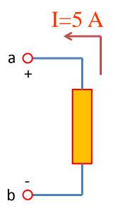
$$V_{ab} = 10 \text{ V}$$
