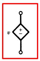
**VCVS: Voltage controlled voltage source**
