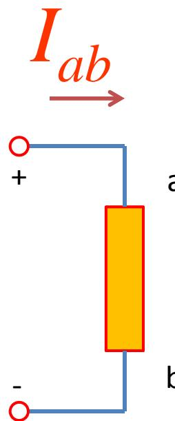
$$P = I_{ab} \times V_{ab}$$
