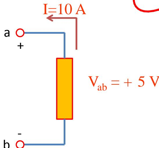
$$P = I_{ab} \times V_{ab}$$
