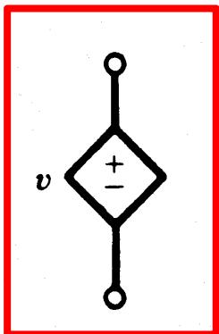
**VCVS: Voltage controlled voltage source**
