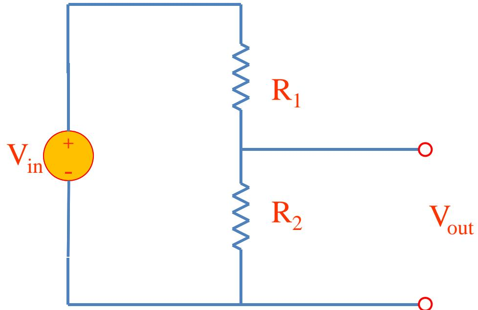
$$V_{out} = \frac{R_1}{R_1 + R_2} V_{in}$$
