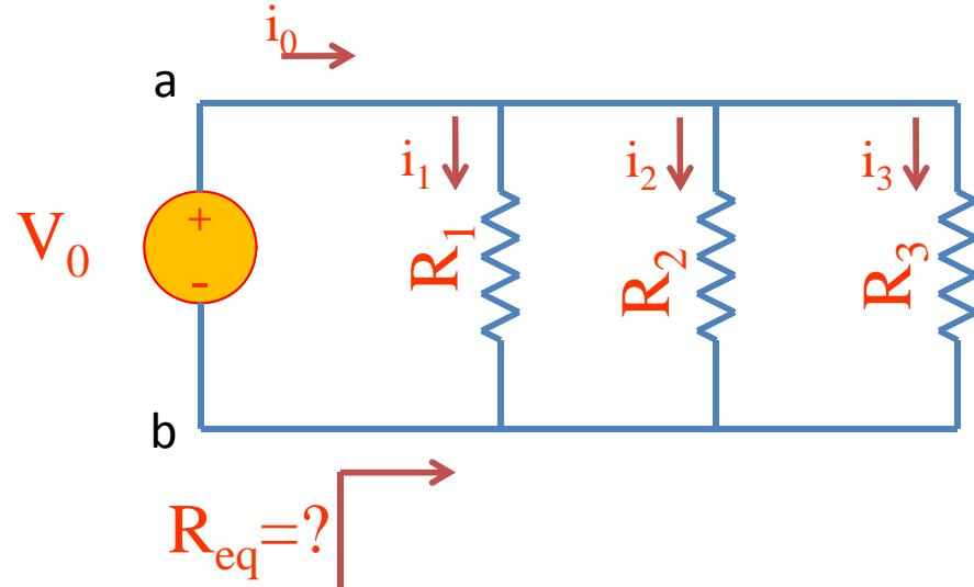
$$a) i_1 = \frac{V_0}{R_1}$$
