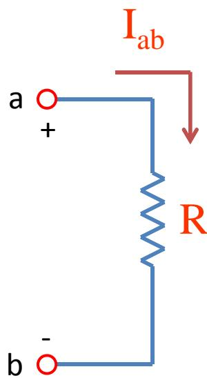
$$V_{ab} = I_{ab} \times R$$
