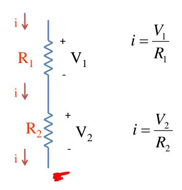
V<sub>1</sub> is the voltage drop across resistor 1
