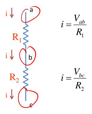
V<sub>ab</sub> is the voltage drop across resistor 1
