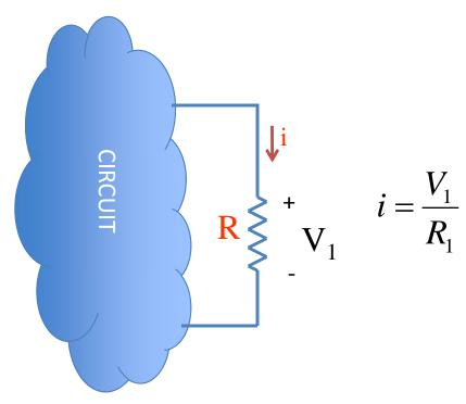
V<sub>1</sub> is the voltage drop across resistor 1
