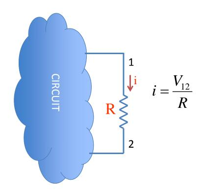
V<sub>12</sub> is the voltage drop across resistor 1
