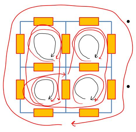
A loop is a closed path with no node passed more than once.
