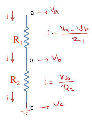
$V_{ab}$  is the voltage drop across resistor 1
