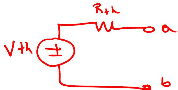
(Monster HW problem: Part 2): Find the Thevenin & Norton equivalent circuit of the circuit below with respect to terminals a and b:
