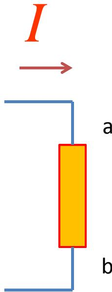
$$I \times V_{ab} = \text{power}$$
