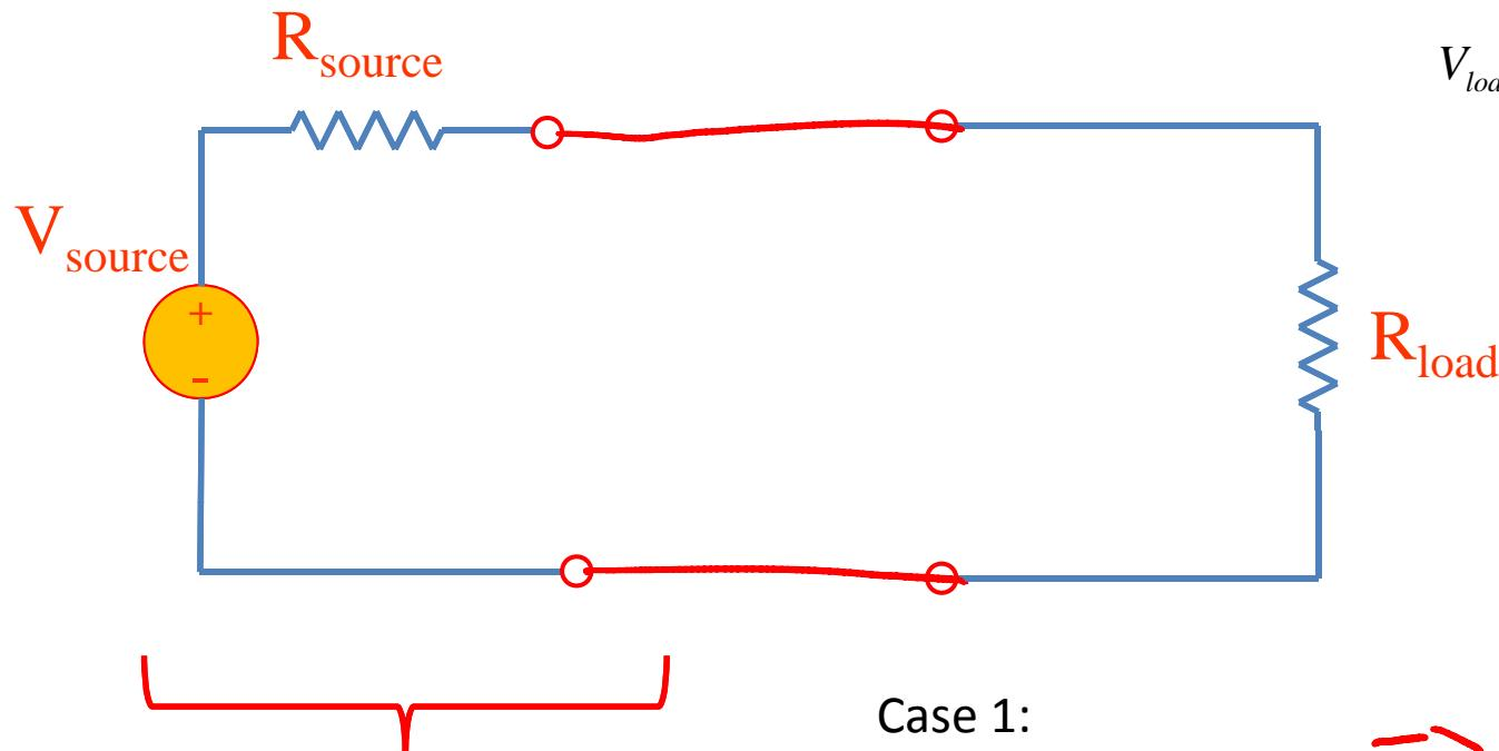
$$V_{load} = \frac{R_{load}}{R_{load} + R_{source}} V_{source}$$
