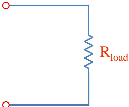
$$V_{load} = \frac{R_{load}}{R_{load} + R_{source}} V_{source}$$
