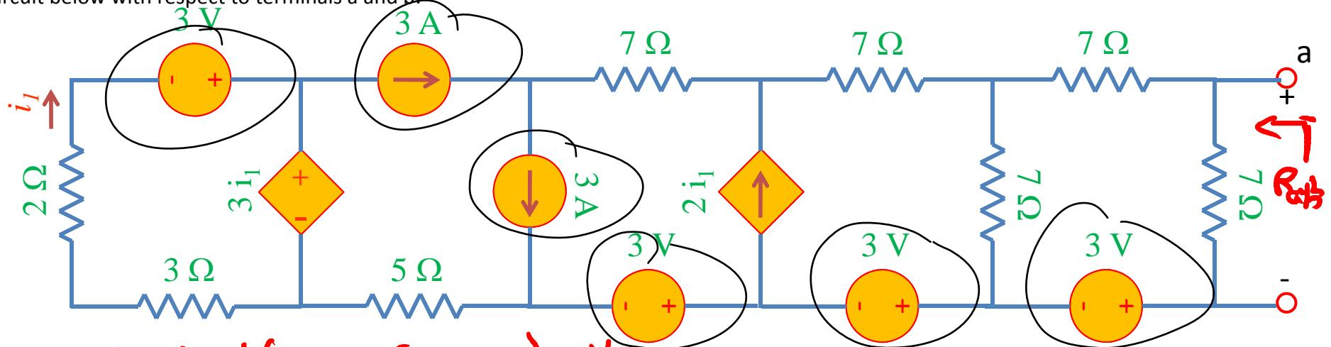
$$1) \text{ Find } V_{ab} (\text{open}) = V_{th}$$
