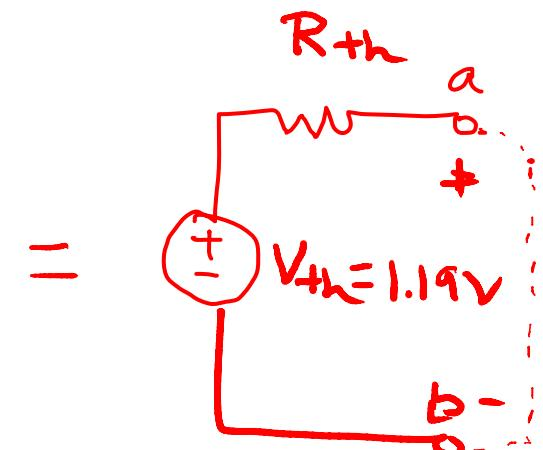
1) Find  $V_{ab}$  complex circuit w/ nothing connected to a,b.
