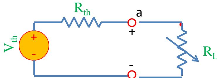
Arrow means  $R_L$  variable (e.g. by a knob)
