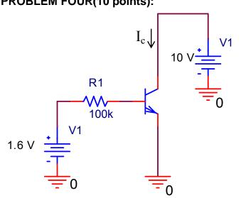
For the amplifier circuit above, assume  $\beta = 1$  and the turn-on voltage for  $V_{BE}$  is 0.6 V. Find the collector current  $I_c$ .
