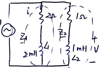
$$Z_1 = 2\Omega + j\omega L_1 = 2\Omega + j \times 1000 \times 2 \times 10^{-3} = 2 + 2j \Omega$$
