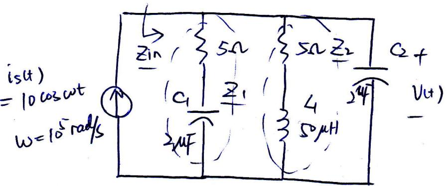
$$\underline{Z_{C_1}} = \frac{1}{j\omega C_1} = \frac{1}{j \times 10^5 \times 2 \times 10^{-6}} = -5j \Omega$$
