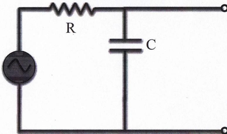
$$\begin{aligned} V_{th} &= V_{oc} = \frac{\frac{1}{j\omega C}}{\frac{1}{j\omega C} + R} \cdot V_s \\ &= \frac{1}{1 + j\omega RC} \cdot V_s \\ &= \frac{V_0}{1 + j\omega RC} \end{aligned}$$
