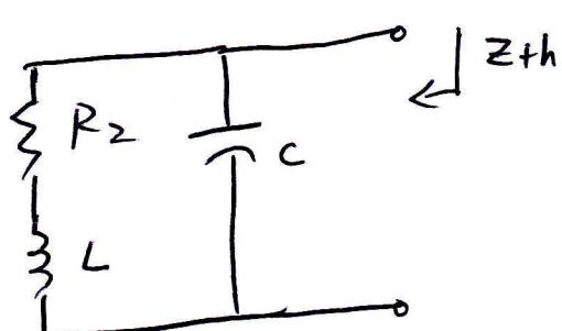
$$\begin{aligned} Z_{th} &= (R_2 + j\omega L) // \frac{1}{j\omega C} \\ &= (2 + 2j) // -2j \\ &= \frac{(2+2j) \cdot (-2j)}{2+2j-2j} \\ &= 2-2j \Omega \end{aligned}$$
