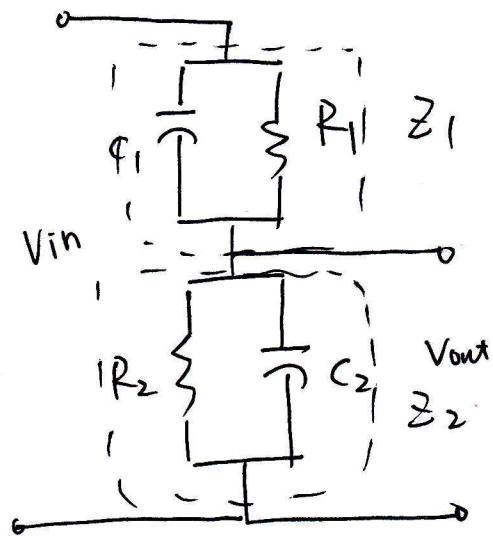
$$Z_1 = R_1 \parallel \frac{1}{j\omega C_1} = \frac{R_1 \cdot \frac{1}{j\omega C_1}}{R_1 + \frac{1}{j\omega C_1}} = \frac{R_1}{1 + j\omega R_1 C_1}$$
