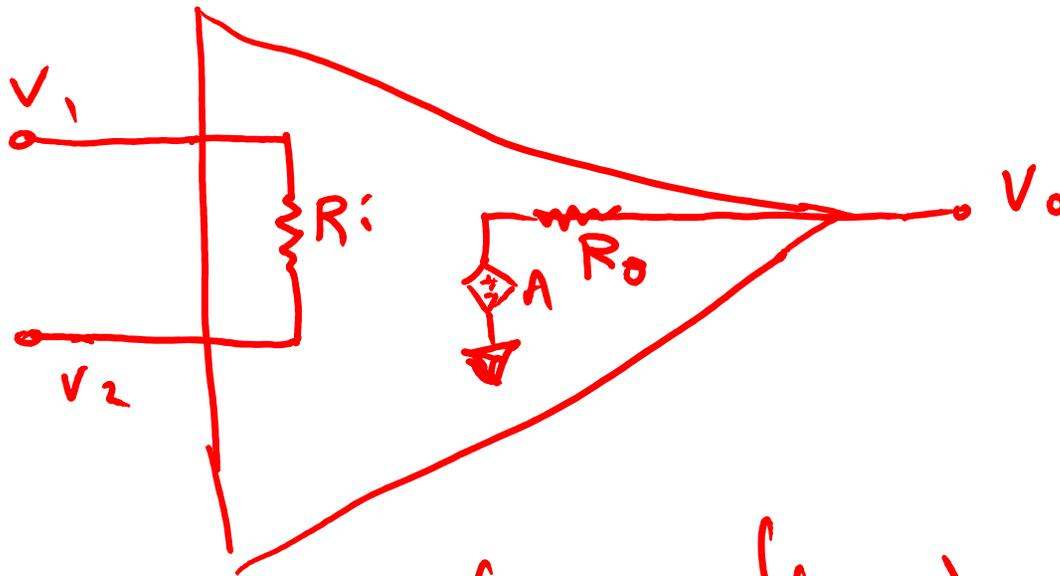
$$V_0 = A (V_2 - V_1)$$
