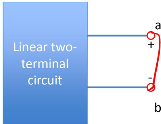
$$V_{a-b} = V_{th} = I_N R_N \quad (*)$$
