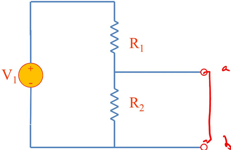
$$1) V_{th} = V_{ab} \text{ (open)}$$
