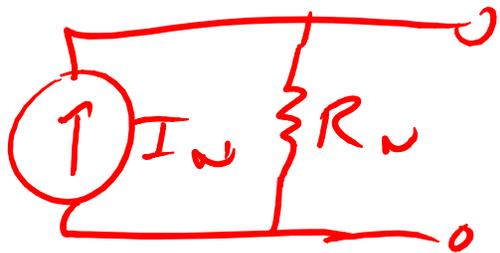
$$R_n = R_1 \parallel R_2 \quad (= R_{th})$$
