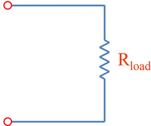
$$V_{load} = \frac{R_{load}}{R_{load} + R_{source}} V_{source}$$
