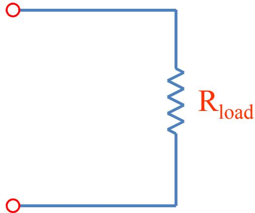
$$V_{load} = \frac{R_{load}}{R_{load} + R_{source}} V_{source}$$
