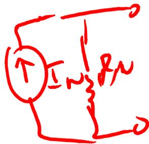
$$= \frac{\frac{V_1 R_2}{R_1 + R_2}}{\frac{V_1}{R_1}} = \frac{R_1 R_2}{R_1 + R_2} = R_1 \parallel R_2$$
