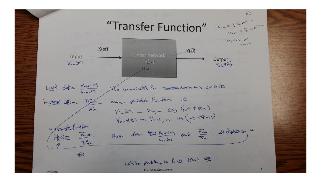
2 Significance of 1/40)  $V_{in}$  (th =  $V_{in}$  , m (os (wt t  $\Phi_{in}$ )  $\overline{V}_{in} = V_{in}$  m  $e^{-i \frac{1}{2} \Phi_{in}}$ Vout(t) = Vout, m (os att Dout) Vout = . Vout e itout H(w) = Vont = Vio Vontin eiton = Vontin eiton Vin = Vin eiton = Vout, m e 's(About - Din) Vin, m |Hews] = Voution tells us importantials above applitude Phose & M(w) = phase shift out is in pour-bir=phose \$1(w)\$ Vorr~= [m) En pour
