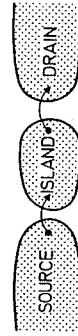
Figure 1. The quantum tunneling of electrons between a "source" and a "drain" electrode through an intermediate "island" electrode can be blocked if the electrostatic energy of a single excess electron on the island is large compared with the energy of thermal fluctuations.
