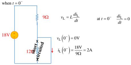
The current across the inductor is continuous  $i_L(0^+) = i_L(0^-)$
