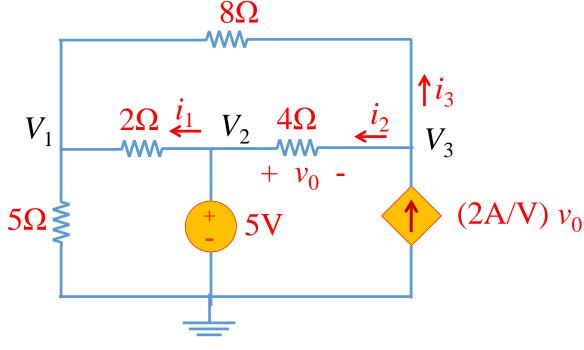
By using node 2 voltage and rearranging the KCL equations
