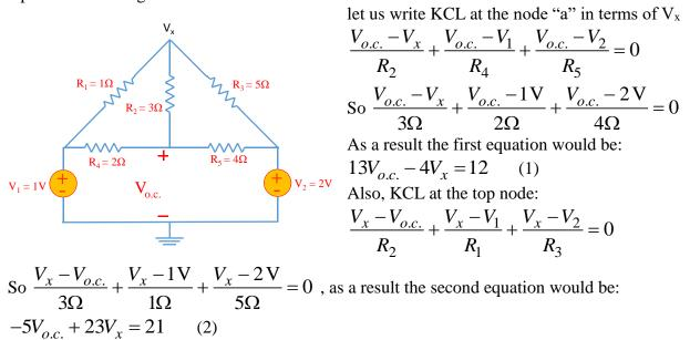
By solving (1) and (2), we reach  $V_x=1.193V$  and  $V_{o.c.}=1.29$  V. So  $v_{Th} = V_{o.c.}=1.29$  V To calculate the  $R_{Th}$ , we kill the independent voltage sources and find the equivalent resistance from a-b terminal:
