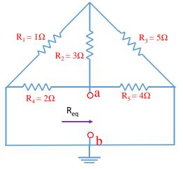
$$\begin{aligned} \mathbf{R}_{\text{Th}} &= \mathbf{R}_{\text{eq}} = [(\mathbf{R}_1 || \mathbf{R}_3) + \mathbf{R}_2] ||(\mathbf{R}_4 || \mathbf{R}_5) \\ &= [(1\Omega || 5\Omega) + 3\Omega] ||(2\Omega || 4\Omega) \\ &= [\frac{5}{6}\Omega + 3\Omega] ||\left(\frac{8}{6}\Omega\right) = \frac{92}{93}\Omega = 0.98\Omega \end{aligned}$$
