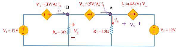
KVL in the left mesh:  $-V_1 - V_3 + V_x = 0$ , So  $V_x - 3i_b = 12$  (1) KVL in the middle mesh:  $-V_x + V_4 + R_7 \cdot i_b = 0$ , So  $-V_x + 15i_b = 0$  (2) By solving (1) and (2), we reach  $i_b = 1$ A and  $V_x = 15$  V To find the powered absorbed/supplied by elements 3, 4 and 5, we need to calculate
