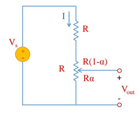
Solution:  $I = V_s / (R + R(1-\alpha) + R\alpha) = V_s / (2R)$   $V_{out} = R\alpha \times I = R\alpha \times V_s / (2R)$ We need  $V_{out} = V_s/3 \rightarrow \alpha = 2/3$
