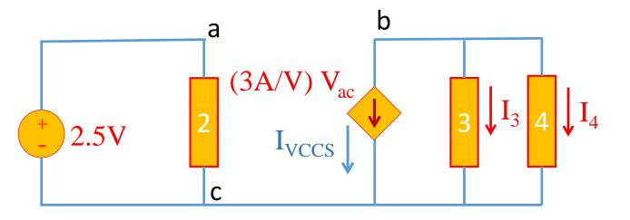
Solution:  $V_{ac} = 2.5V$ VCCS current =  $I_{VCCS} = (3A/V) V_{ac} = 7.5A$ KCL @ node b:  $I_3 + I_4 + I_{VCCS} = 0$  $\Rightarrow I_3 + I_4 = -7.5A$  Problem 2: (CCVS/CCCS) Find I<sub>1</sub>, I<sub>2</sub> and V<sub>bc</sub>
