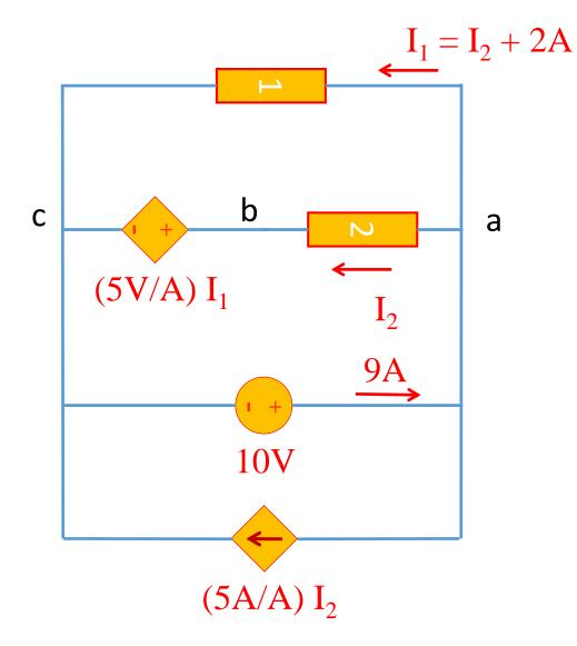
Solution:  $V_{ac} = 2.5 V$ KCL @ node a:  $I_1 + I_2 - 9A + 5I_2 = 0$ From the question we know  $I_1 = I_2 + 2A$  $\rightarrow I_2 = 1 A$ ,  $I_1 = 3 A$ ,  $V_{bc} = 5I_1 = 5 V$  Problem 3: (VCVS) Find  $V_{bc}$  and  $V_{ab}$ .
