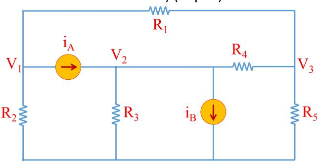
Solution. Write KCL for all three nodes of the circuit:
