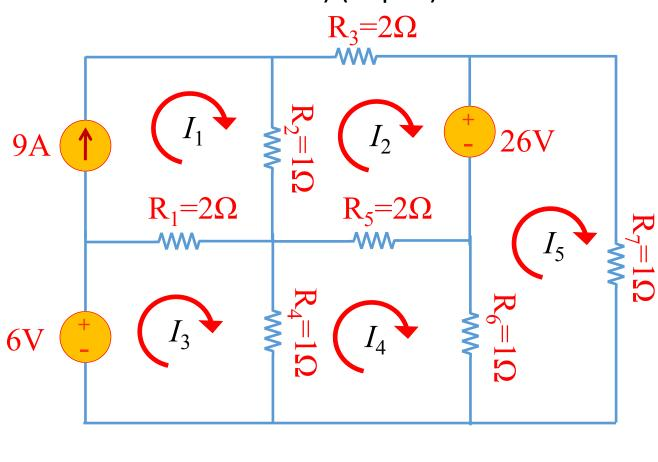
Solution. Write KVL for loops I<sub>2</sub> through I<sub>5</sub>:
