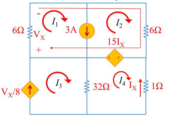
Solution: Note we have a current source in the loop 1, we have a "supermesh" in this circuit, reducing the number of the equations.
