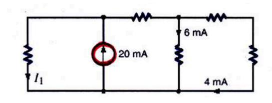
KCL at mode B:  $I_2 = Gm + 4m$   $I_2 = 10m A$ KCL at mode A:  $I_1 + I_2 = 20m$   $I_1 = 20m - 10m$  $I_1 = 10m A$
