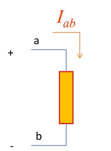
$V_{ab}$  positive =>  $V_a$  >  $V_b$  $I_{ab}$  positive => current flows from a to b  $V_{ab}$  negative =>  $V_a$  <  $V_b$
