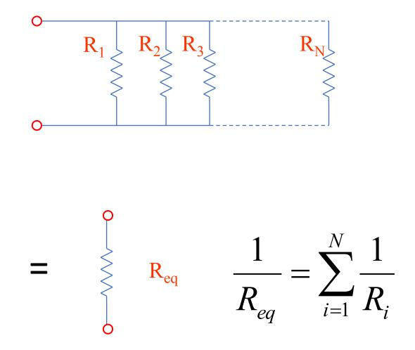
$R_1 \parallel R_2$  is notation for " $R_1$  in parallel with  $R_2$ "
