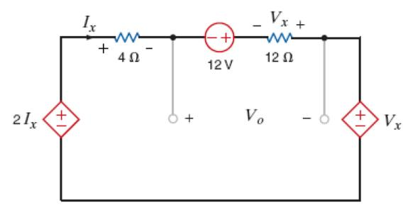
KVL.  $V_0 + 12 + V_x = 0$  $V_0 = -V_x - 12$  $V_x = -12 T_x$
