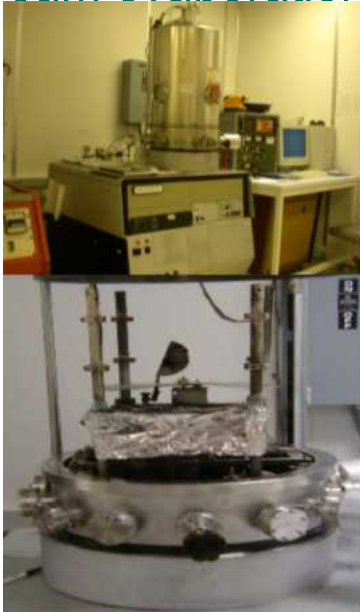
Electron beam evaporator
