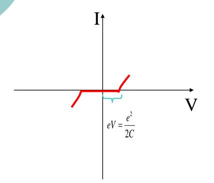
From quantum circuit theory, works even when voltage biased.
