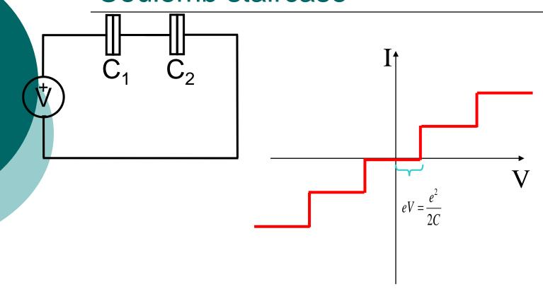
Overall slope is R<sub>tunnel</sub>, which is *large*.
