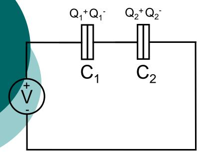
$$Q_1 = \frac{C_1(C_2V - Q_i)}{C_1 + C_2}$$
