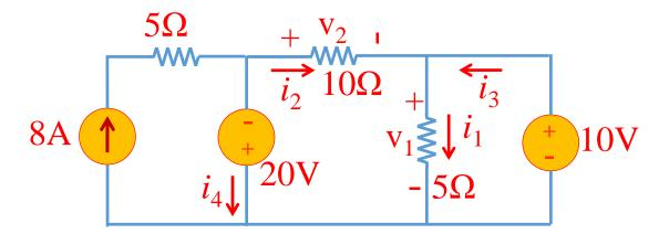
Problem 2: Use nodal analysis and find  $V_1$  through  $V_4$  and  $i_1$  through  $i_4$  (10pts.)
