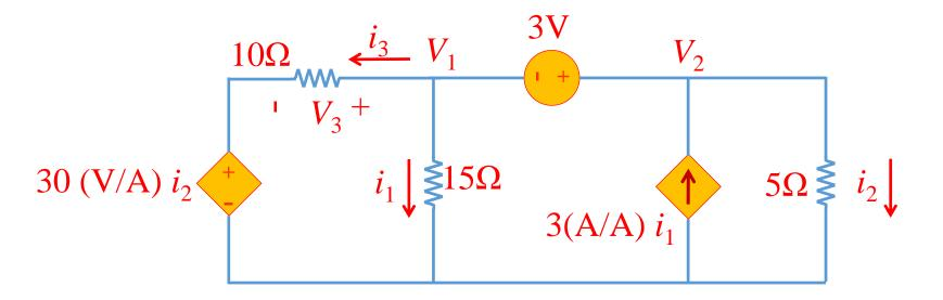
Problem 4: Write all nodal voltage equations and put them in the matrix form (you do not need to solve for voltages  $V_1$  through  $V_4$ ) (10pts.)
