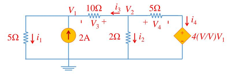
Problem 3: Use nodal analysis and find  $V_1$  through  $V_3$  and  $i_1$  through  $i_3$  (10pts.)
