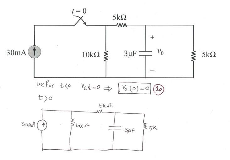
to find time constant Z=RC, we need to find the Resistance seen from the terminals of capacitor while canceling independent voltage and current sources. (make independ voltage source wire, make independent current source open)
