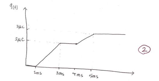
Problem 4: The current flowing through the in the inductor is given as a function of time in the following figure. Plot the voltage of the inductor,  $V_L(t)$ . Mark the axis of your plot with numbers and units. (5pts)
