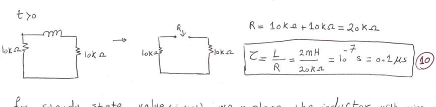
for steady state value (i\_(\infty)), we replace the inductor with wire or short circuit to
